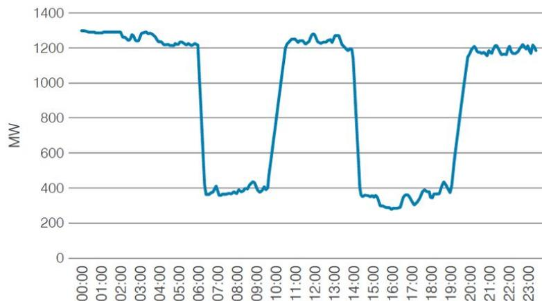
Most of the nuclear reactors in France can reduce their power twice a day, every day, going down to 20% of nominal power in half an hour. However, this theoretical capability is not always used. On average, a reactor performs 15 variations per year, but this figure is increasing because more and more renewable electricity is being injected into the grid.
